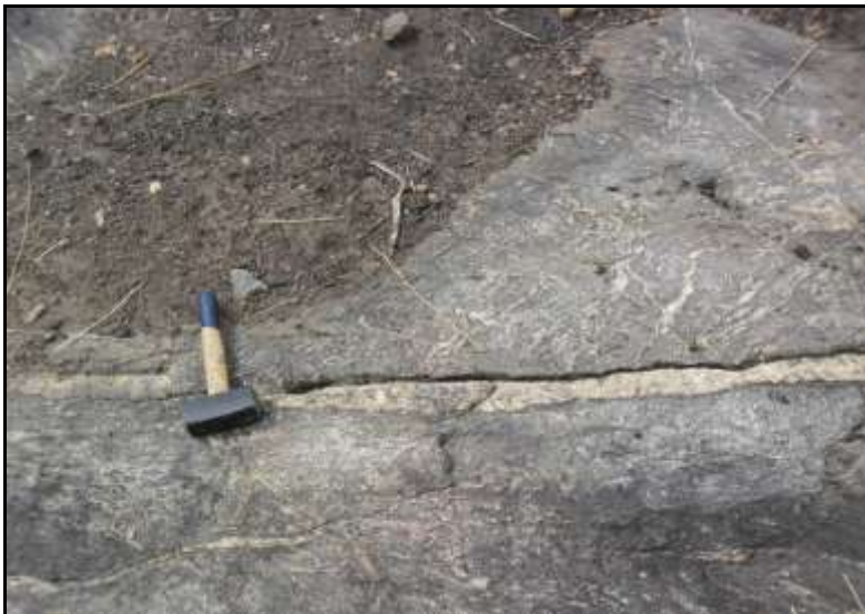
Figure 26: A fracture in migmatitic gneiss healed with quartzo-feldspatic materials (06°59'06"N, 09°26'38"E).
